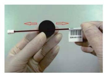
FIGURE 6A. Capillary mixing.
