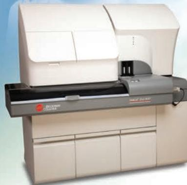
With the DxI 800, operators can load reagents and similar consumables 'on the fly', without using the console computer, minimizing manual intervention.
